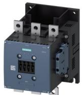
power contactor, AC-3e/AC-3 265 A, 132 kW / 400 V without operating mechanism 3-pole, auxiliary contacts 2 NO + 2 NC main circuit: busbar control and auxiliary circuit: screw terminal
