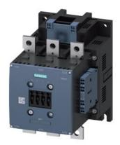
power contactor, AC-3e/AC-3 300 A, 160 kW / 400 V, AC (50-60 Hz) / DC Uc: 220-240 V 3-pole, auxiliary contacts 2 NO + 2 NC drive: conventional main circuit: busbar control and auxiliary circuit: spring-loaded terminal
