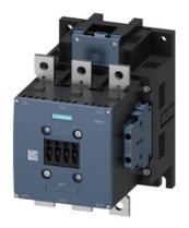
power contactor, AC-3e/AC-3 300 A, 160 kW / 400 V, AC (50-60 Hz) / DC Uc: 96-127 V PLC input 24 V DC 3-pole, auxiliary contacts 2 NO + 2 NC drive: electronic main circuit: busbar control and auxiliary circuit: screw terminal
