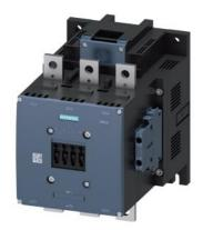
power contactor, AC-3e/AC-3 500 A, 250 kW / 400 V AC (50-60 Hz) / DC Uc: 440-480 V 3-pole, auxiliary contacts 2 NO + 2 NC drive: conventional main circuit: busbar control and auxiliary circuit: screw terminal
