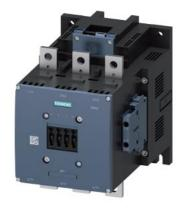
power contactor, AC-3e/AC-3 500 A, 250 kW / 400 V AC (50-60 Hz) / DC Uc: 21-27.3 V PLC input 24 V DC 3-pole, auxiliary contacts 2 NO + 2 NC drive: electronic main circuit: busbar control and auxiliary circuit: screw
