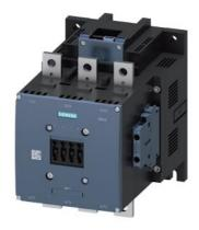
power contactor, AC-3e/AC-3 500 A, 250 kW / 400 V AC (50-60 Hz) / DC Uc: 96-127 V PLC input 24 V DC 3-pole, auxiliary contacts 2 NO + 2 NC drive: electronic main circuit: busbar control and auxiliary circuit: screw terminal
