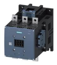
power contactor, AC-3e/AC-3 500 A, 250 kW / 400 V AC (50-60 Hz) / DC Uc: 200-277 V PLC input 24 V DC 3-pole, auxiliary contacts 2 NO + 2 NC drive: electronic main circuit: busbar control and auxiliary circuit: screw terminal
