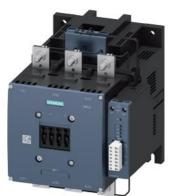
power contactor, AC-3e/AC-3 500 A, 250 kW / 400 V AC (50-60 Hz) / DC Uc: 96-127 V PLC input 24 V DC 3-pole, auxiliary contacts 1 NO + 1 NC drive: electronic main circuit: busbar control and auxiliary circuit: screw terminal with remaining lifetime indicator
