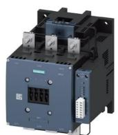
power contactor, AC-3e/AC-3 500 A, 250 kW / 400 V AC (50-60 Hz) / DC Uc: 200-277 V PLC input 24 V DC 3-pole, auxiliary contacts 1 NO + 1 NC drive: electronic main circuit: busbar control and auxiliary circuit: screw terminal with remaining lifetime indicator
