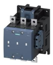
vacuum contactor AC-3e/AC-3 225 A, 110 kW / 400 V, 3-pole, Uc: 23-26 V AC(50-60 Hz) / DC drive: conventional auxiliary contacts 2 NO + 2 NC main circuit: busbar control and auxiliary circuit: screw terminal
