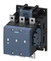
vacuum contactor AC-3e/AC-3 225 A, 110 kW / 400 V, 3-pole, Uc: 110-127 V AC(50-60 Hz) / DC drive: conventional auxiliary contacts 2 NO + 2 NC main circuit: busbar control and auxiliary circuit: screw terminal
