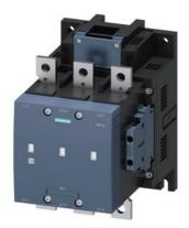
vacuum contactor AC-3e/AC-3 225 A, 110 kW / 400 V, 3-pole, Uc: 200-220 V AC(50-60 Hz) / DC drive: conventional auxiliary contacts 2 NO + 2 NC main circuit: busbar control and auxiliary circuit: screw terminal
