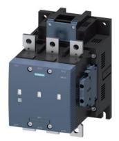
vacuum contactor AC-3e/AC-3 225 A, 110 kW / 400 V, 3-pole, Uc: 440-480 V AC(50-60 Hz) / DC drive: conventional auxiliary contacts 2 NO + 2 NC main circuit: busbar control and auxiliary circuit: screw terminal
