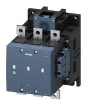
vacuum contactor AC-3e/AC-3 225 A, 110 kW / 400 V, 3-pole, Uc: 96-127 V AC(50-60 Hz) / DC PLC input 24 V DC drive: electronic auxiliary contacts 2 NO + 2 NC main circuit: busbar control and auxiliary circuit: screw terminal
