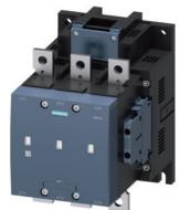
vacuum contactor AC-3e/AC-3 265 A, 132 kW / 400 V, 3-pole, Uc: 42-48 V AC(50-60 Hz) / DC drive: conventional auxiliary contacts 2 NO + 2 NC main circuit: busbar control and auxiliary circuit: screw terminal
