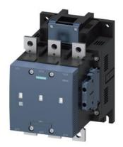
vacuum contactor AC-3e/AC-3 265 A, 132 kW / 400 V, 3-pole, Uc: 110-127 V AC(50-60 Hz) / DC drive: conventional auxiliary contacts 2 NO + 2 NC main circuit: busbar control and auxiliary circuit: screw terminal
