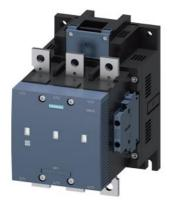
vacuum contactor AC-3e/AC-3 265 A, 132 kW / 400 V, 3-pole, Uc: 220-240 V AC(50-60 Hz) / DC drive: conventional auxiliary contacts 2 NO + 2 NC main circuit: busbar control and auxiliary circuit: screw terminal
