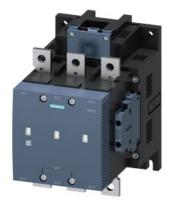
vacuum contactor AC-3e/AC-3 265 A, 132 kW / 400 V, 3-pole, Uc: 21-27.3 V AC(50-60 Hz) / DC PLC input 24 V DC drive: electronic auxiliary contacts 2 NO + 2 NC main circuit: busbar control and auxiliary circuit: screw terminal
