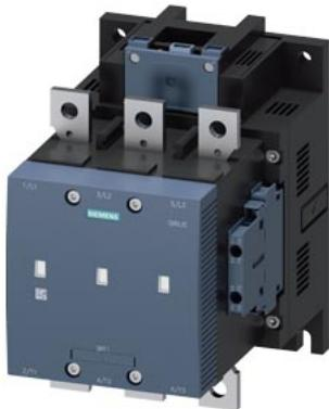
vacuum contactor AC-3e/AC-3 265 A, 132 kW / 400 V, 3-pole, Uc: 200-277 V AC(50-60 Hz) / DC PLC input 24 V DC drive: electronic auxiliary contacts 2 NO + 2 NC main circuit: busbar control and auxiliary circuit: screw terminal
