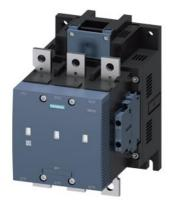
vacuum contactor AC-3e/AC-3 300 A, 160 kW / 400 V, 3-pole, Uc: 23-26 V AC(50-60 Hz) / DC drive: conventional auxiliary contacts 2 NO + 2 NC main circuit: busbar control and auxiliary circuit: screw terminal
