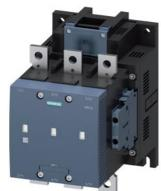
vacuum contactor AC-3e/AC-3 300 A, 160 kW / 400 V, 3-pole, Uc: 42-48 V AC(50-60 Hz) / DC drive: conventional auxiliary contacts 2 NO + 2 NC main circuit: busbar control and auxiliary circuit: screw terminal
