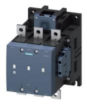
vacuum contactor AC-3e/AC-3 300 A, 160 kW / 400 V, 3-pole, Uc: 21-27.3 V AC(50-60 Hz) / DC PLC input 24 V DC drive: electronic auxiliary contacts 2 NO + 2 NC main circuit: busbar control and auxiliary circuit: screw terminal
