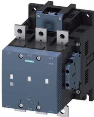
vacuum contactor AC-3e/AC-3 300 A, 160 kW / 400 V, 3-pole, Uc: 200-277 V AC(50-60 Hz) / DC PLC input 24 V DC drive: electronic auxiliary contacts 2 NO + 2 NC main circuit: busbar control and auxiliary circuit: screw terminal
