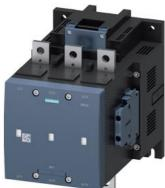
vacuum contactor AC-3e/AC-3 400 A, 200 kW / 400 V, 3-pole, Uc: 23-26 V AC(50-60 Hz) / DC drive: conventional auxiliary contacts 2 NO + 2 NC main circuit: busbar control and auxiliary circuit: screw terminal
