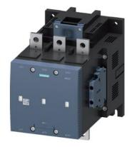
vacuum contactor AC-3e/AC-3 400 A, 200 kW / 400 V, 3-pole, Uc: 42-48 V AC(50-60 Hz) / DC drive: conventional auxiliary contacts 2 NO + 2 NC main circuit: busbar control and auxiliary circuit: screw terminal
