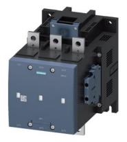
vacuum contactor AC-3e/AC-3 400 A, 200 kW / 400 V, 3-pole, Uc: 240-277 V AC(50-60 Hz) / DC drive: conventional auxiliary contacts 2 NO + 2 NC main circuit: busbar control and auxiliary circuit: screw terminal
