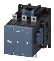
vacuum contactor AC-3e/AC-3 400 A, 200 kW / 400 V, 3-pole, Uc: 380-420 V AC(50-60 Hz) / DC drive: conventional auxiliary contacts 2 NO + 2 NC main circuit: busbar control and auxiliary circuit: screw terminal
