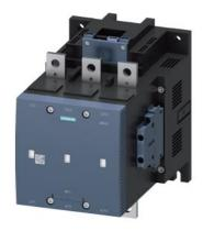
vacuum contactor AC-3e/AC-3 400 A, 200 kW / 400 V, 3-pole, Uc: 200-277 V AC(50-60 Hz) / DC PLC input 24 V DC drive: electronic auxiliary contacts 2 NO + 2 NC main circuit: busbar control and auxiliary circuit: screw
