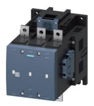
vacuum contactor AC-3e/AC-3 500 A, 250 kW / 400 V, 3-pole, Uc: 23-26 V AC(50-60 Hz) / DC drive: conventional auxiliary contacts 2 NO + 2 NC main circuit: busbar control and auxiliary circuit: screw terminal
