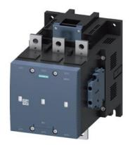
vacuum contactor AC-3e/AC-3 500 A, 250 kW / 400 V, 3-pole, Uc: 42-48 V AC(50-60 Hz) / DC drive: conventional auxiliary contacts 2 NO + 2 NC main circuit: busbar control and auxiliary circuit: screw terminal
