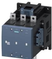
vacuum contactor AC-3e/AC-3 500 A, 250 kW / 400 V, 3-pole, Uc: 500-550 V AC(50-60 Hz) / DC drive: conventional auxiliary contacts 2 NO + 2 NC main circuit: busbar control and auxiliary circuit: screw terminal
