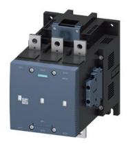
vacuum contactor AC-3e/AC-3 500 A, 250 kW / 400 V, 3-pole, Uc: 575-600 V AC(50-60 Hz) / DC drive: conventional auxiliary contacts 2 NO + 2 NC main circuit: busbar control and auxiliary circuit: screw terminal
