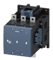
vacuum contactor AC-3e/AC-3 500 A, 250 kW / 400 V, 3-pole, Uc: 200-277 V AC(50-60 Hz) / DC PLC input 24 V DC drive: electronic auxiliary contacts 2 NO + 2 NC main circuit: busbar control and auxiliary circuit: screw terminal
