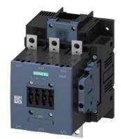
power contactor AC-1 275 A / 690 V / 40  $^\circ$ C 3-pole, Uc: 500-550 V AC(50-60 Hz) / DC drive: conventional auxiliary contacts 2 NO + 2 NC main circuit: busbar control and auxiliary circuit: screw terminal
