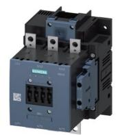
power contactor AC-1 275 A / 690 V / 40  $^\circ$ C 3-pole, Uc: 240-277 V AC(50-60 Hz) / DC drive: conventional auxiliary contacts 2 NO + 2 NC main circuit: busbar control and auxiliary circuit: screw terminal
