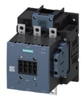
power contactor AC-1 275 A / 690 V / 40 °C 3-pole, Uc: 380-420 V AC(50-60 Hz) / DC drive: conventional auxiliary contacts 2 NO + 2 NC main circuit: busbar control and auxiliary circuit: screw terminal
