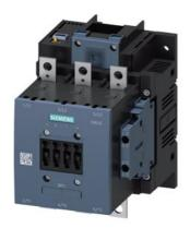
power contactor AC-1 275 A / 690 V / 40  $^{\circ}$ C 3-pole, Uc: 21-27.3 V AC(50-60 Hz) / DC PLC input 24 V DC drive: electronic auxiliary contacts 2 NO + 2 NC main circuit: busbar control and auxiliary circuit: screw terminal
