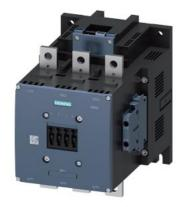
power contactor AC-1 690 A / 690 V / 40  $^{\circ}$ C 3-pole, Uc: 96-127 V AC(50-60 Hz) / DC PLC input 24 V DC drive: electronic auxiliary contacts 2 NO + 2 NC main circuit: busbar control and auxiliary circuit: screw terminal
