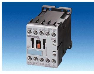
CONTACTOR, AC-3 4 KW/400 V, AC-1 18 A, CC 24 V 50/60 HZ, 4-POLE, 2 NO + 2 NC, SIZE S00, SCREW CONNECTION
