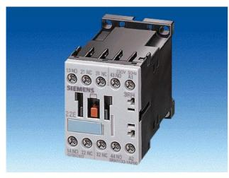
CONTACTOR, AC-3 4 KW/400 V, AC-1 18 A, AC 230V 50/60HZ, 4-POLE, 2 NO + 2 NC, SIZE S00, SCREW CONNECTION
