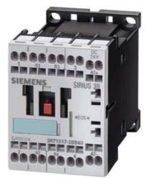
CONTACTOR, AC-3 5.5KW/400 V, AC-1, 22 A, DC 24 V, 4-POLE, 2 NO + 2 NC, SIZE S00, CAGE-CLAMP CONNECTION
