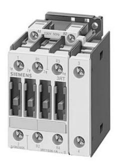
CONTACTOR, AC-3, 11KW/400V, DC 24 V, 4-POLE, 2 NO + 2 NC, SIZE S0, SCREW CONNECTION
