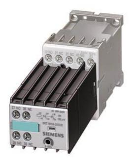
SOLID-STATE, TIME-DELAYED AUXILIARY SWITCH BLOCK SETTING RANGE 0.5 S...10 S AC 100...127 V, 1NO + 1NC, ON-DELAY, FOR MOUNTING ONTO CONTACTORS SIZES00
