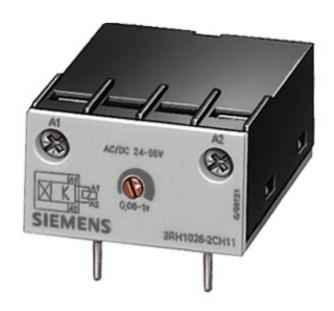
SOLID-STATE TWO-WIRE TIME RELAY SETTING RANGE 0.5 S...10 S, AC/DC 24...66 V, ON-DELAY, WITH VARISTOR FOR MOUNTING ONTO CONTACTORS SIZE S0...S3
