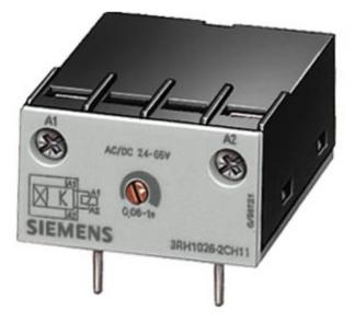
SOLID-STATE TWO-WIRE TIME RELAY SETTING RANGE 5 S...100 S, AC/DC 90...240 V, ON-DELAY, WITH VARISTOR, FOR MOUNTING ONTO CONTACTORS SIZE S0...S3
