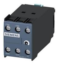
solid-state time-delayed front-side auxiliary switch Time range 0.05...1 s,  $100 \dots 127 \text{ V AC}$ , 1 NO contact, 1 NC contact ON delay, for 3RT1
