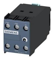
solid-state time-delayed front-side auxiliary switch Time range 0.5...10 s,  $100 \dots 127 \text{ V AC}$ , 1 NO contact, 1 NC contact ON delay, for 3RT1
