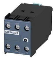
solid-state time-delayed front-side auxiliary switch Time range 5...100 s, 100 ... 127 V AC, 1 NO contact, 1 NC contact ON delay, for 3RT1
