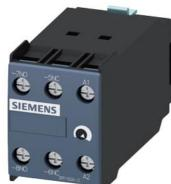
solid-state time-delayed front-side auxiliary switch Time range 0.5...10 s, 24 V AC/DC, 1 NO contact, 1 NC contact OFF delay, without control signal for 3RT1
