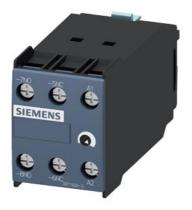
solid-state time-delayed front-side auxiliary switch Time range 0.05...1 s, 100 ... 127 V AC / DC, 1 NO contact, 1 NC contact OFF delay, without control signal for 3RT1
